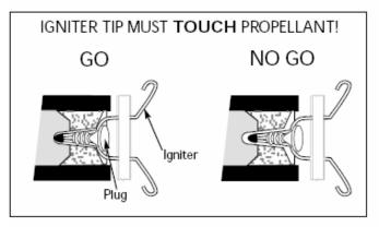
About 90% of all problems with engine ignition are caused by the igniter not being properly and securely held in place in the engine.
